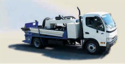
**General Specifications:** Type: Swing tube model with dual reciprocating pistons.
